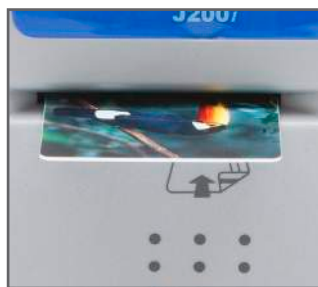
Front loading card feed
