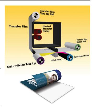
• Zebra's patented image transfer process applies film to both sides of the card in a single pass, drastically reducing the print time.
